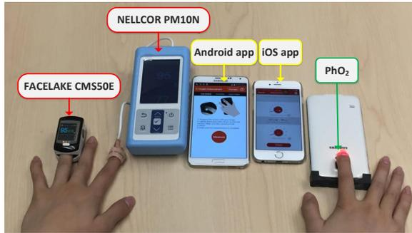
**Figure 10: Experiment setup to compare PhO<sub>2</sub> with other 4 pulse oximeters**
